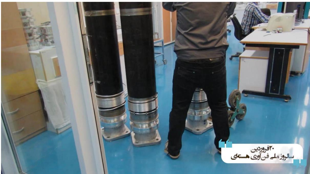
**Figure 14.** The image is a view of the bottom half of recipients and their base, showing the cooling water coils around the bottom of the recipient. The cooling is used to remove surplus heat from the rotor and to set up the temperature gradient along the rotor to stimulate the internal uranium hexafluoride gas flow. Stacks of motor housings may be visible in the left top of the top photo.
