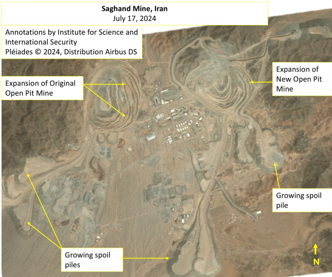
Figure 4. The Saghand mine underwent notable expansion in the last years; first, a new open pit mine was added, then, both open pit mines were expanded. Top: Saghand in 2022; bottom: Saghand in July 2024.
