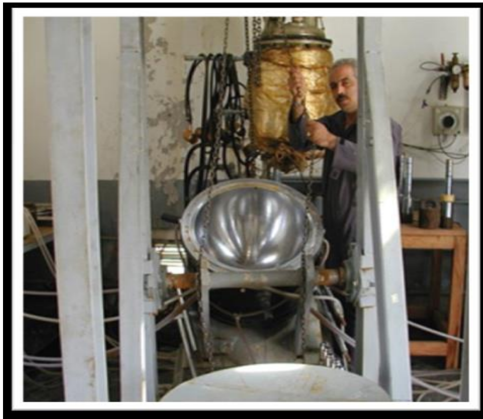
Figure 3. Image from the Nuclear Archive that shows a high explosive casting mold at an unidentified location in Iran. The equipment in the background could not be identified.
