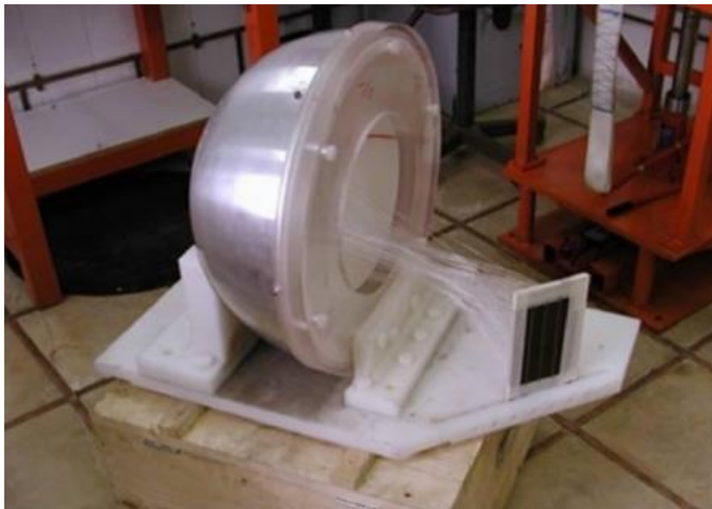
Figure 8. Model of an experimental system in the Nuclear Archive representing what appears to be a shock wave generator and high explosives, with a diagnostic system using fiber optic cables, to measure time of arrival of a detonation front in the main charge.
