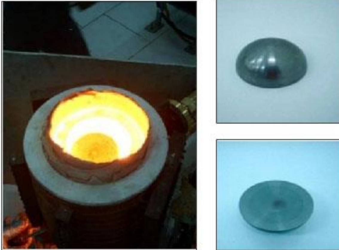
Figure 14. Molten material, along with cast hemispheres, in the pilot plant, Iranian images from the Nuclear Archive. It is not clear what type of surrogate material is in these images from the archive, based on the information available to the Institute.
