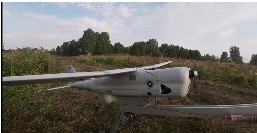
Figure 1. A screenshot from a demonstration video of an Orlan-10 UAV on its launch catapult.
