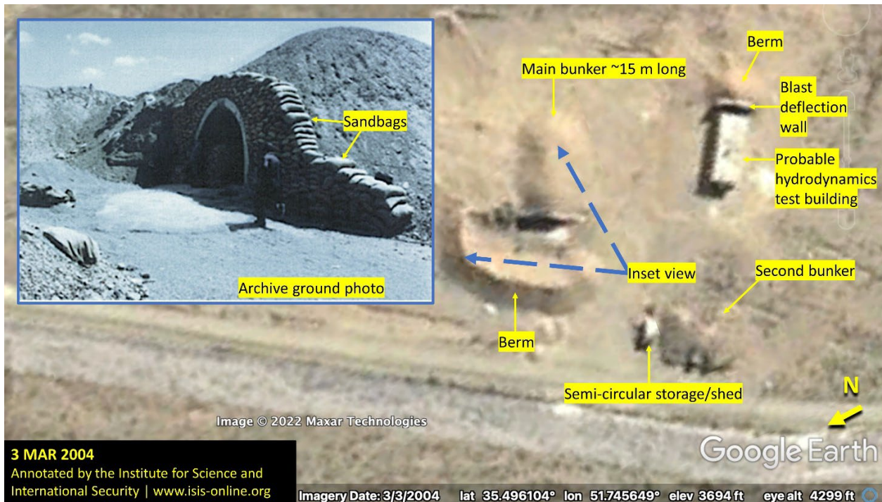
Figure 8. The Golab Dareh site in March 2004 featured a large bunker and a building suitable for nuclear-weapons related testing and developing high-speed diagnostic equipment.
