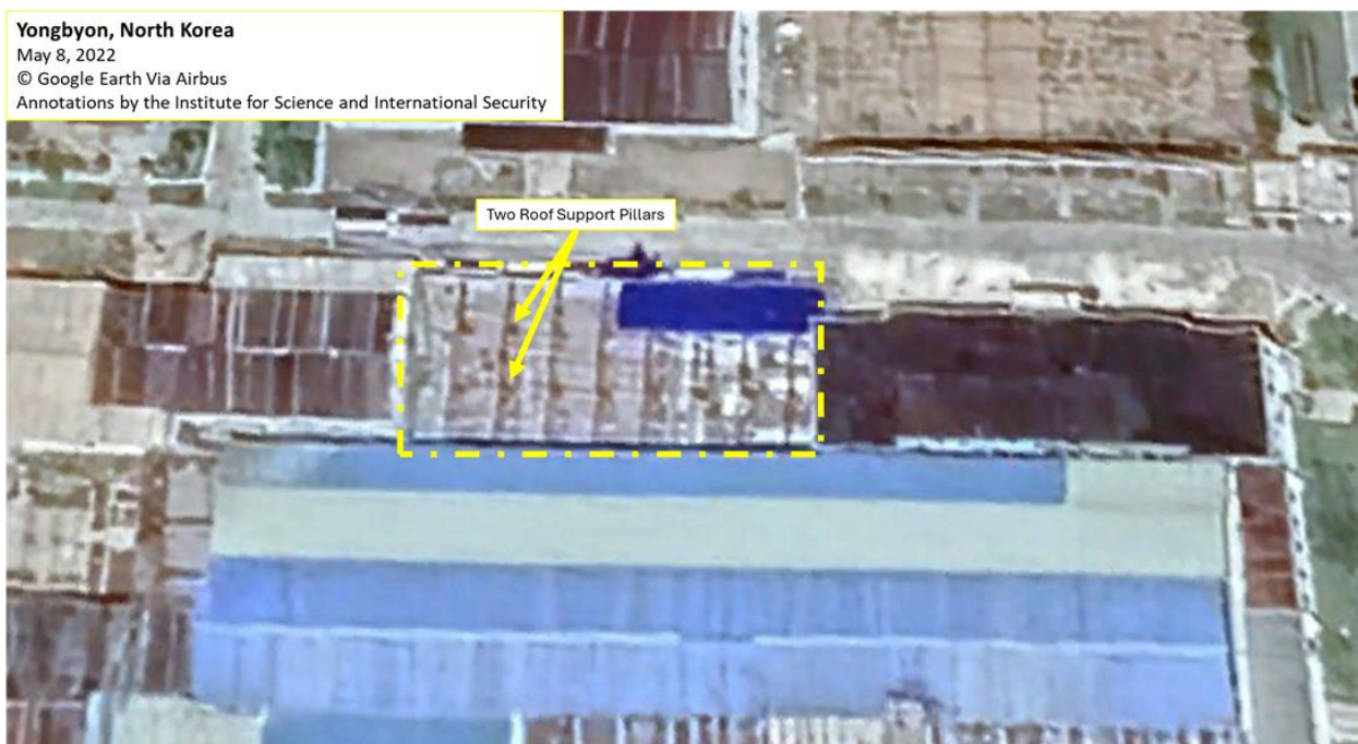
Figure 24. A Google Earth image of the construction of the annex at Yongbyon. The image shows the internal structure of the room. Two roof support pillars are visible, as seen in a January 2025 ground image.
