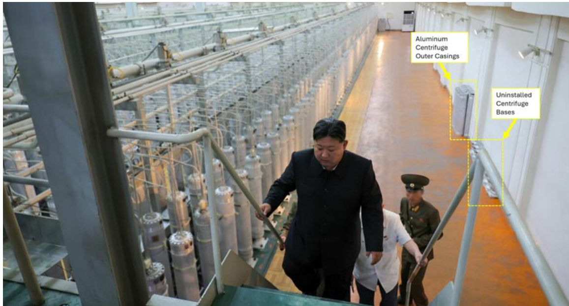
Figure 8. An image of Kim Jong Un ascending the stairs to the bridge; four centrifuge cascades can be seen, with three on one side of the columns. Noticeably, the columns are on the left-hand side of the image, suggesting the three cascades in Figure 7 are on the other side of the columns, for a total of at least six cascades on one side of the bridge.
