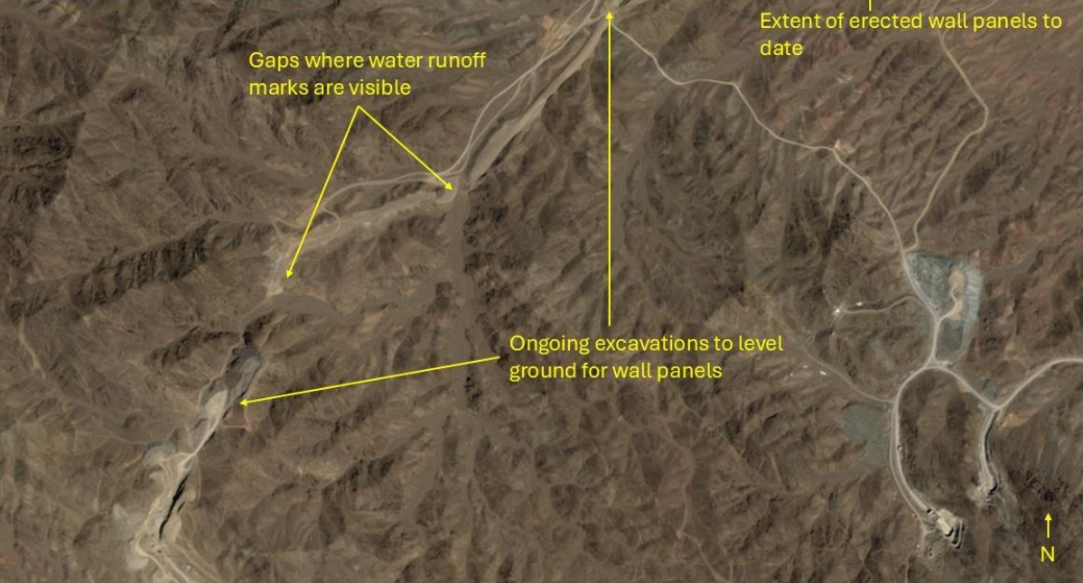
Figure 3. The northwest portion of the perimeter is undergoing road grading and installation of wall panels.
