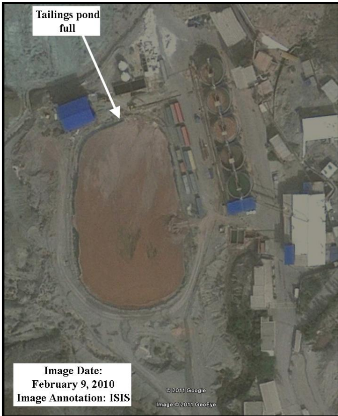
Figure 3. Tailings pond full in February 9, 2010 image of the Gchine uranium mine and mill
