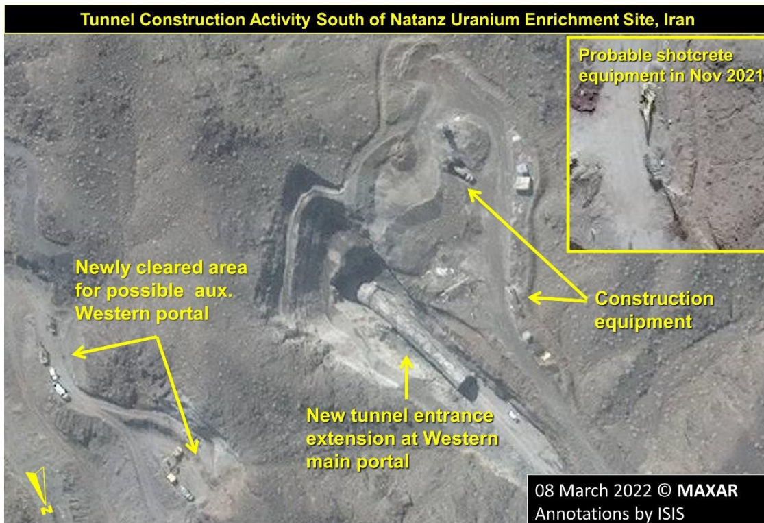
Figure 3. The western tunnel entrance also features a new entrance extension, likely to be covered by earth in the future, as of March 2022.
