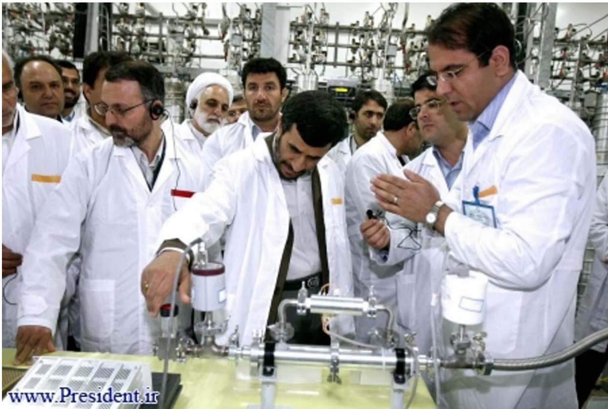
Figure 2: President Ahmadinejad examines gas centrifuge equipment, which includes an older MKS pressure transducer (next to his right hand) during a visit to the Natanz pilot fuel enrichment plant in 2008. In the background is an IR-1 gas centrifuge cascade which contains many more recent (mid-2000s) models of MKS pressure transducers. Source: Website archive of the president of Iran, www.President.ir
