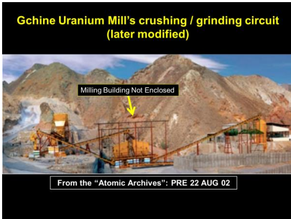
Figure 4. A close-up image from the Nuclear or Atomic Archive showing the milling building before it was enclosed.
