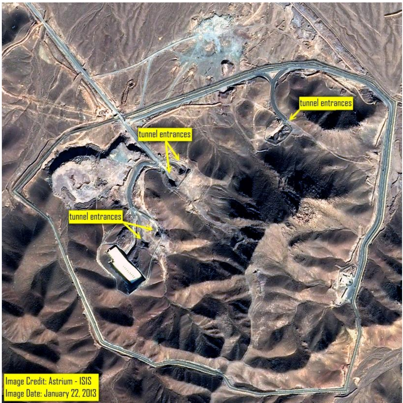
Figure 1. Satellite imagery of the Fordow fuel enrichment site from January 22 nd , one day after the reported explosion that caused major damage to the site. The imagery shows no damage to the exterior and no discernible signs of emergency vehicles or activity at the tunnel entrances.
