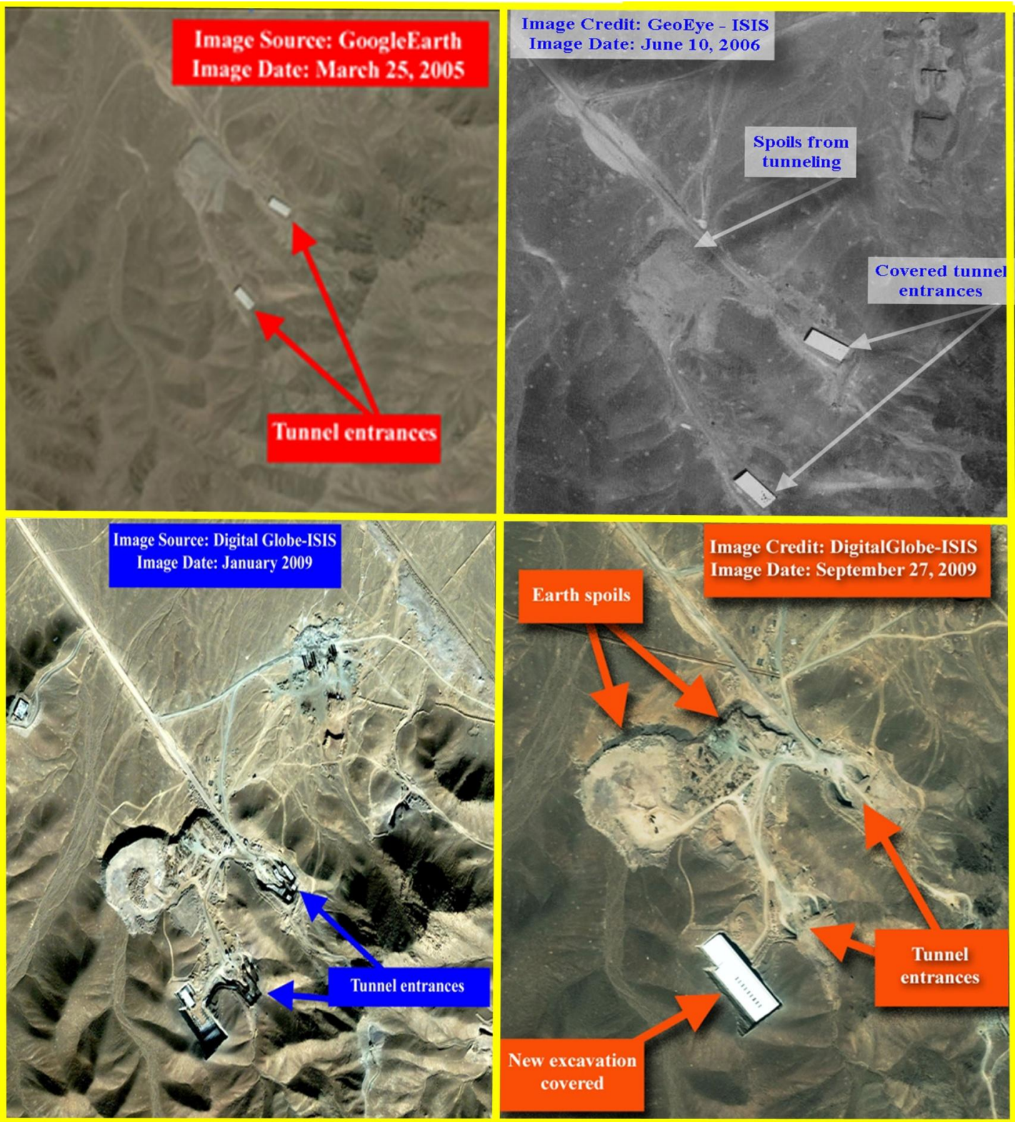
Figure 2. Google Earth/GeoEye/Digital Globe imagery showing the evolution of the Fordow Fuel Enrichment Plant between March 2005 and September 2009.
