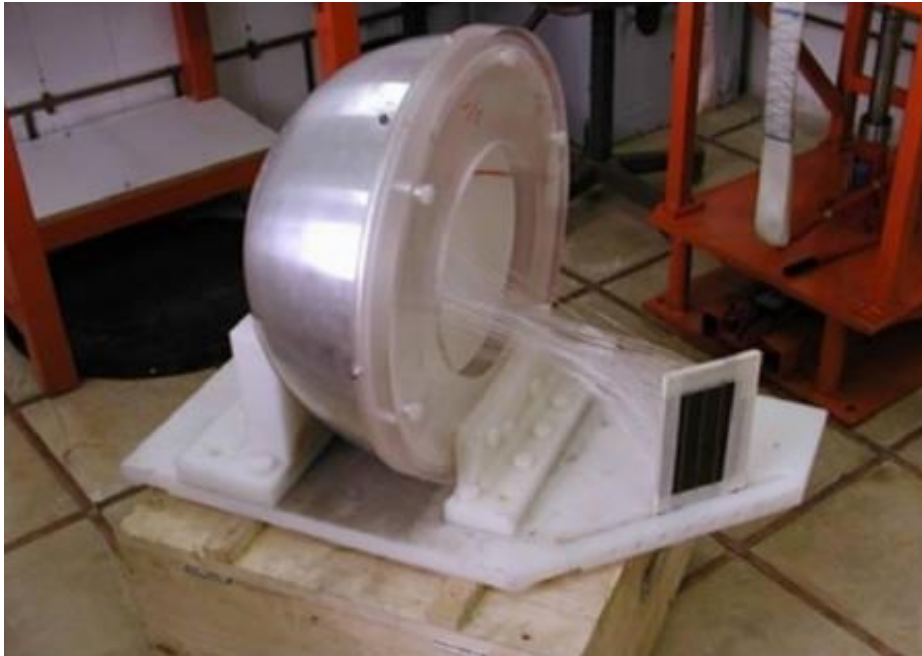
Figure 6. A model of an experimental system in the Nuclear Archive representing what appears to be a shock wave generator and high explosives, with a diagnostic system using fiber optic cables, to measure the time of arrival of a detonation front on the inside edge of the main charge. Such experiments were performed.
