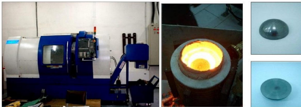
Figure 5. The left image is a computer numerically controlled machine tool that was in Amad's Shahed Mahallati Uranium Metals Workshop and is likely still available to a crash program today. The right collection of three images shows molten material along with cast hemispheres in the pilot plant. Source: Nuclear Archive.
