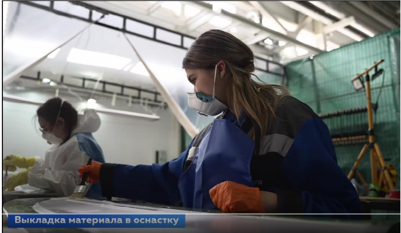
Figure 3. Alabuga Polytechnic participants producing the composite airframe for the Albatross M5 drone. Source: An Alabuga Polytechnic video posted to its Youtube.com channel ( https://www.youtube.com/watch?v=AMHD4pBn5no&t=4s ).
