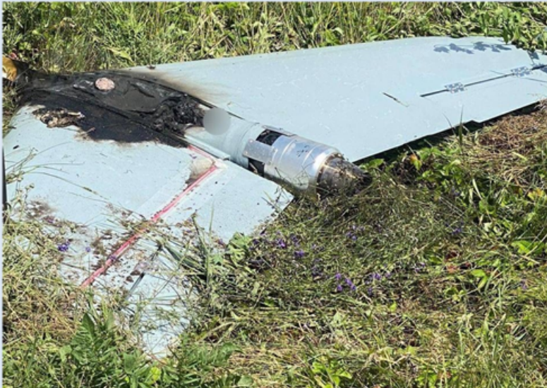
Figure S1. A new, unidentified jet drone shot down on August 30, 2024, was made according to an aerodynamic scheme like Shahed, with no warhead. Source: Defense Express c
