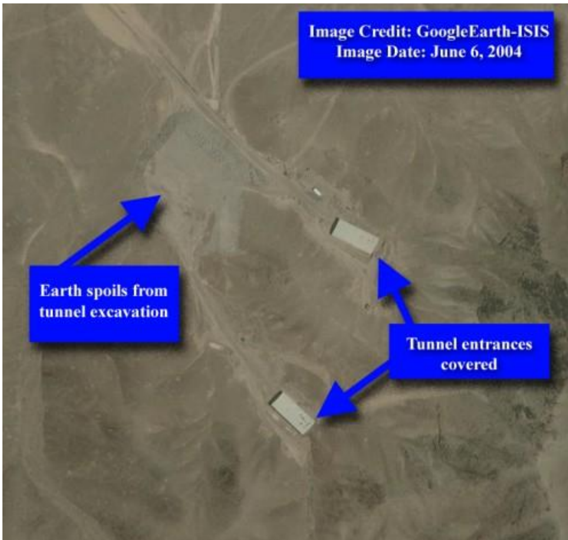
Figure 4. The covered tunnel entrances of the enrichment plant as of June 6, 2004. See also Figure 3.
