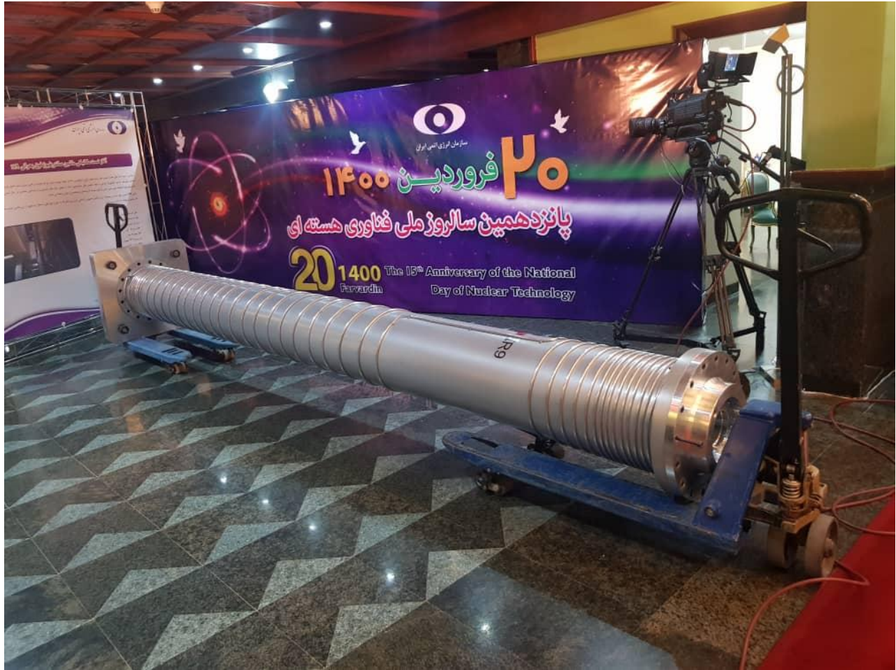
Figure 1.25. IR-9 centrifuge outer casing. The IR-9 centrifuge is still in an early development stage. Source: AEOL, https://aeoi.org.ir/en/portal/home/?news/45799/69280/316331/the-basis-of-this-national-industry-are-meticulously-preserved6
