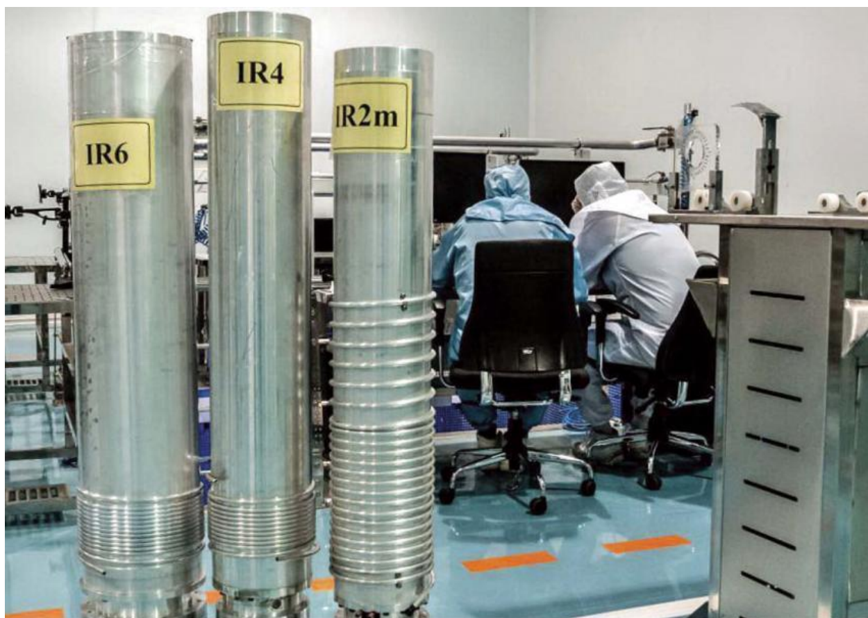
Figure 1.11. IR-2m centrifuge outer casing on right, compared to the IR-6 and IR-4 centrifuge casings. Source: Iran Press News Agency
