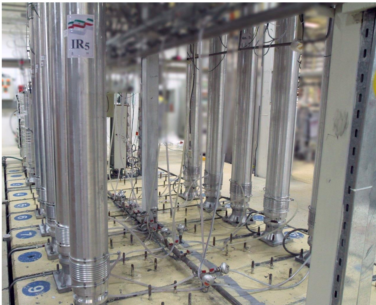
Figure 1.17. Ten IR-5 centrifuges in a small cascade in the Natanz pilot plant. Lines 2 and 3 at the PFEP contained IR-5 centrifuges and other advanced centrifuges, which are visible in the left line of centrifuges, one of which is likely an IR-2m centrifuge. The reason for the blurring of the image is unknown. Source: AEOI
