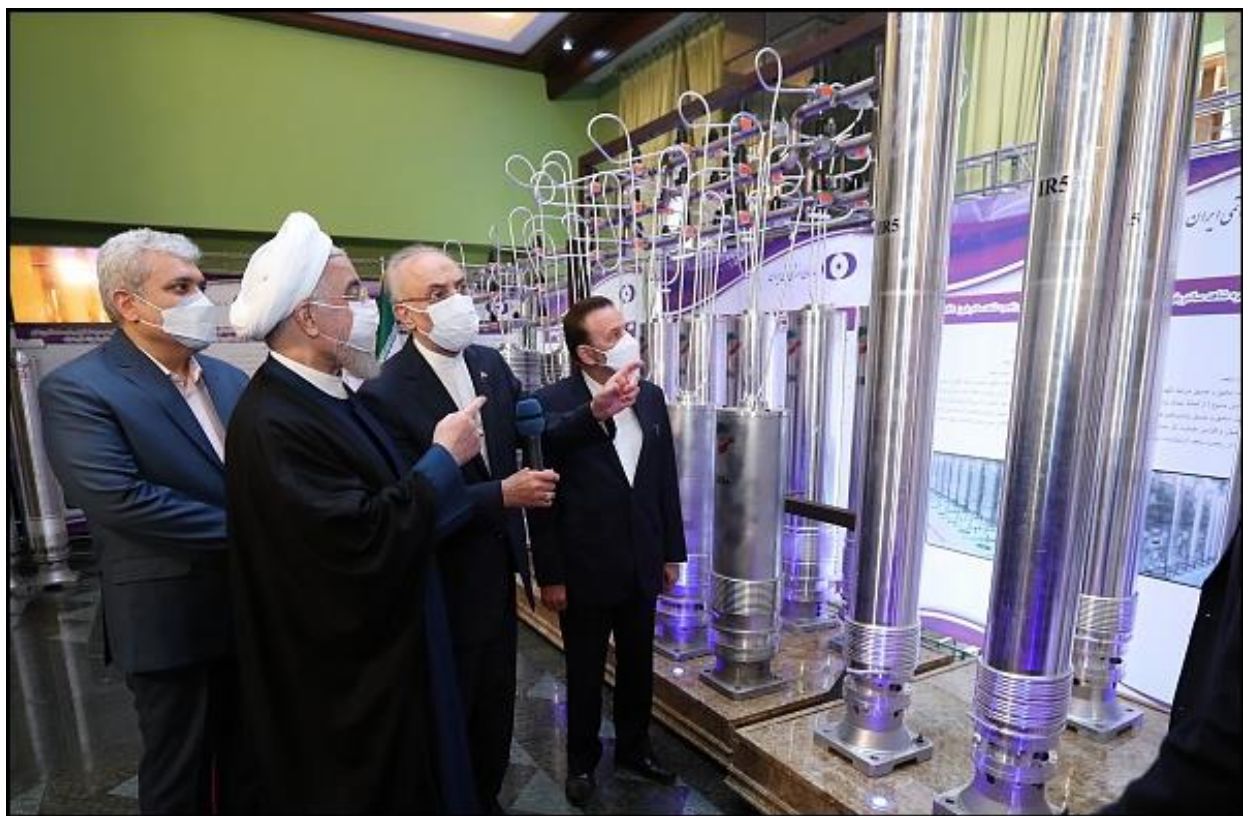
Figure 1.16. IR-5 centrifuges next to much shorter IR-6s and IR-6 centrifuges. These centrifuges appear to be the same ones as in Figure 1.15 but from a different angle. Source: https://president.ir/en/120598
