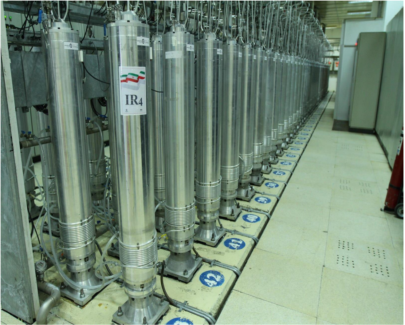
Figure 1.14. A cascade of IR-4 centrifuges at the PFEP. Source: AEOI, see https://aeoi.org.ir/en/portal/home/?news/45799/69280/294523/dr.-salehi-describes-advanced-nuclear-industry-achievements
