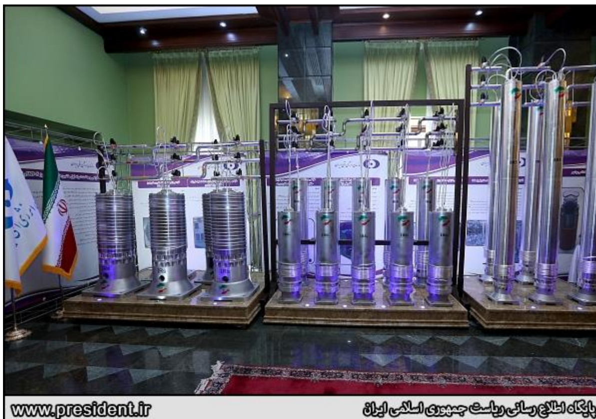
Figure 1.24. Display on Iran's National Nuclear Technology Day in Tehran, April 10, 2021. From left to right: IR-s, IR-6s (front), IR-6 (back), and IR-5 centrifuges, during Iran's National Nuclear Technology Day in Tehran, Iran April 10, 2021. Source: Iranian President's web site, https://president.ir/en/120598
