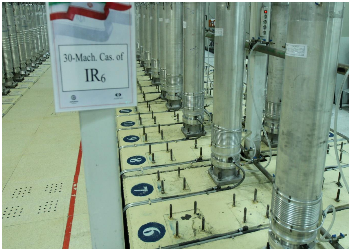
Figure 1.18. IR-6 centrifuges in a cascade at the Natanz pilot plant. Source: AEOL, https://aeoi.org.ir/en/portal/home/?news/45799/69280/294523/dr.-salehi-describes-advanced-nuclear-industry-achievements
