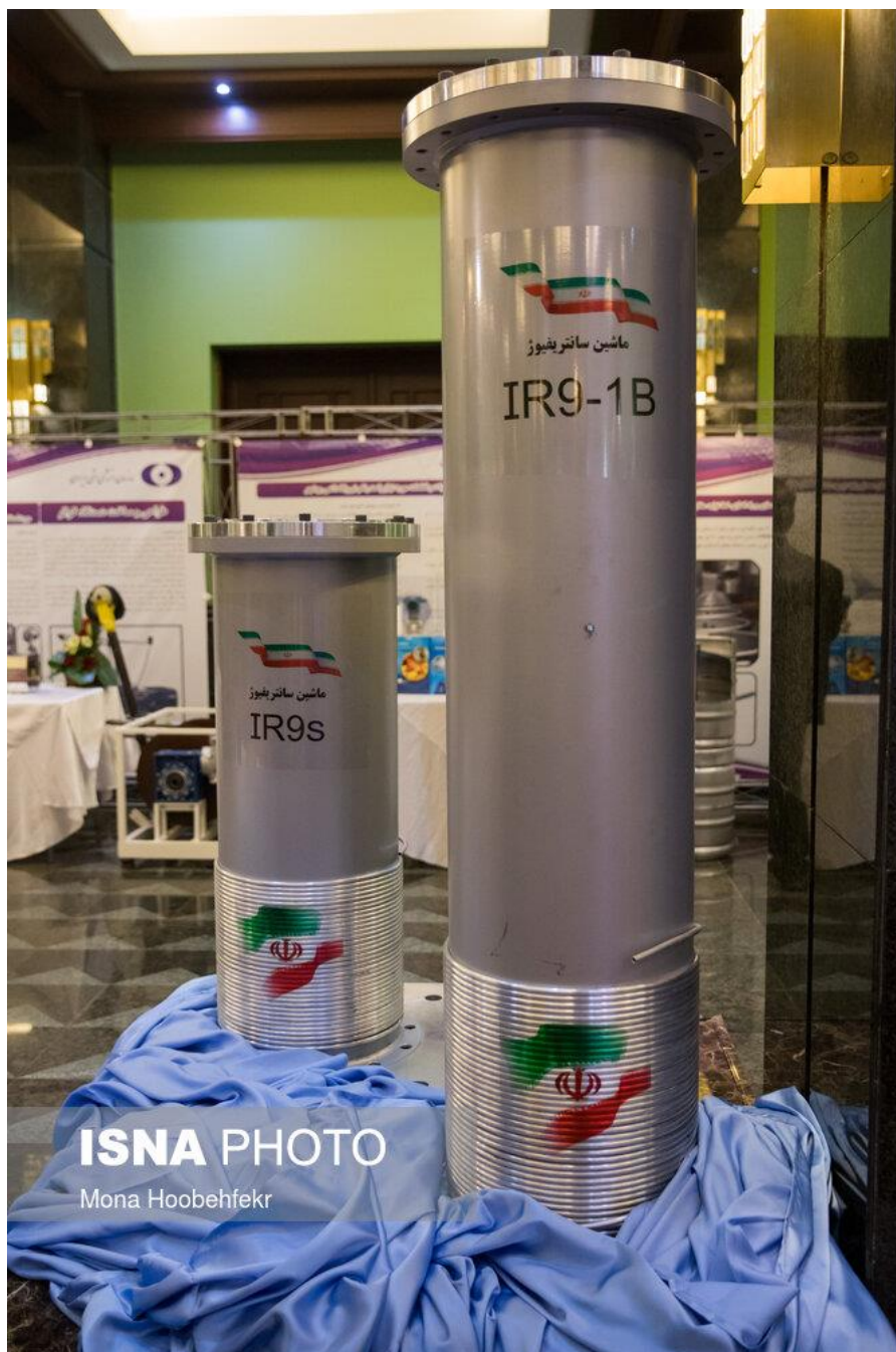
Figure 1.26. Variants of the IR-9 centrifuge (IR-9s and IR9-1B) showing their outer casings. Source: ISNA Photo.
