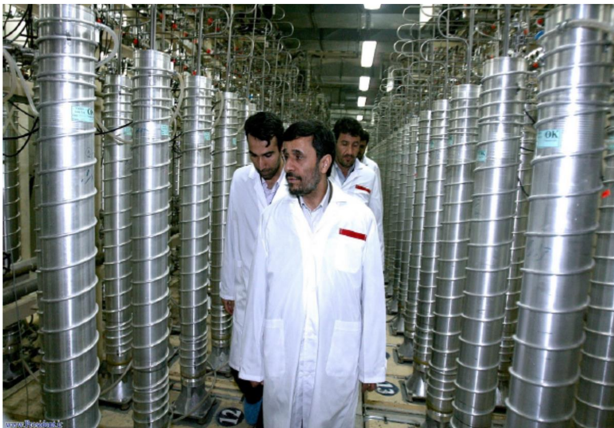
Figure 1.7. IR-1 centrifuge cascades in the Pilot Fuel Enrichment Plant in 2008 during a visit by then President Mahmoud Ahmadinejad.
