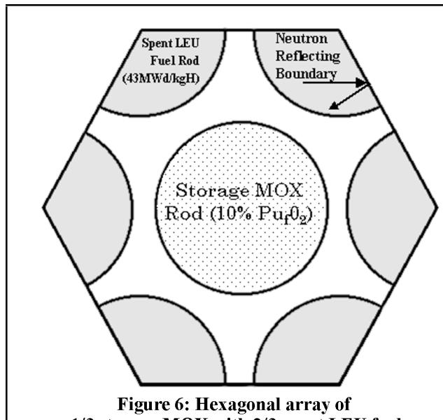
**Figure 6:** Hexagonal array of 1/3 storage MOX with 2/3 spent LEU fuel
