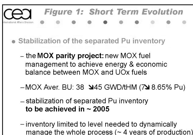
Currently, MOX fuel is licensed in France for three in-core cycles only; that is, a 3-batch reload scheme, which is the same schedule originally used for uranium oxide fuel. To take advantage of the rise in the authorized uranium fuel average burn up from 33 to 48 gigawatt-days per tonne (GWd/t), EDF adopted an hybrid reload strategy—a scheme that uses a 4-batch reload for uranium fuel, and just a 3-batch reload for MOX fuel. This strategy is obviously not optimal.
