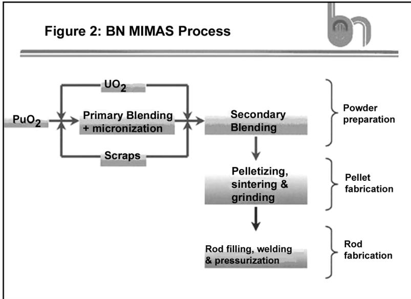
Belgonucleaire started industrial MOX production in 1986, and since then has produced over 420 tonnes of MOX. This corresponds to over 220,000 fuel rods, with which over 800 PWR and almost 300 BWR fuel assemblies have been produced. A total of 64 reloads have been introduced into reactors, and 23 tonnes of plutonium have been recycled this way. It is important to know that there have been no fuel rod failures due to fabrication.
