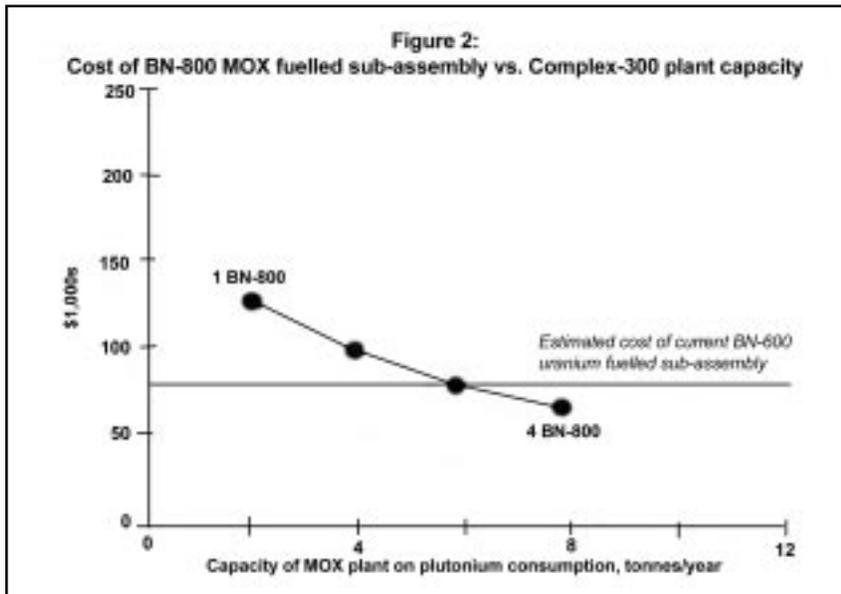
The horizontal line is the existing price to produce uranium fuel. You can see that if there is very low capacity, the price is several times larger compared to uranium fuel.
