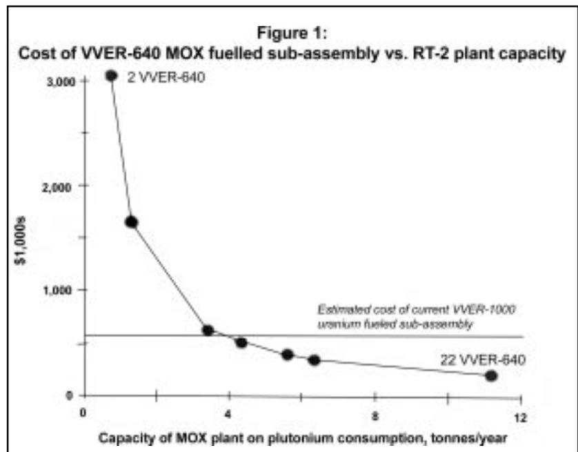
the price of MOX fuel production depends greatly on the capacity of the MOX fuel production plant. The X-axis, along the bottom, is the capacity of the MOX fuel production plant, and the Y-axis is the cost of MOX fuel production.
