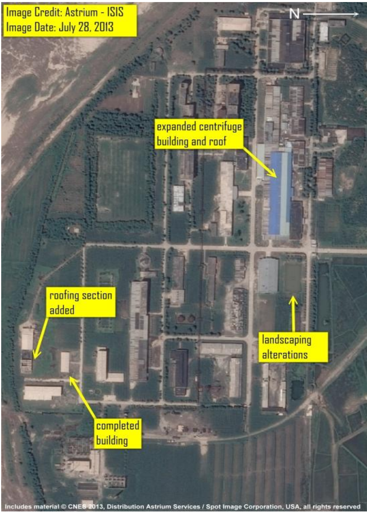
Figure 1. Satellite imagery of the Yongbyon Fuel Fabrication plant from July 28, 2013 showing the expansion of the gas centrifuge plant building.
