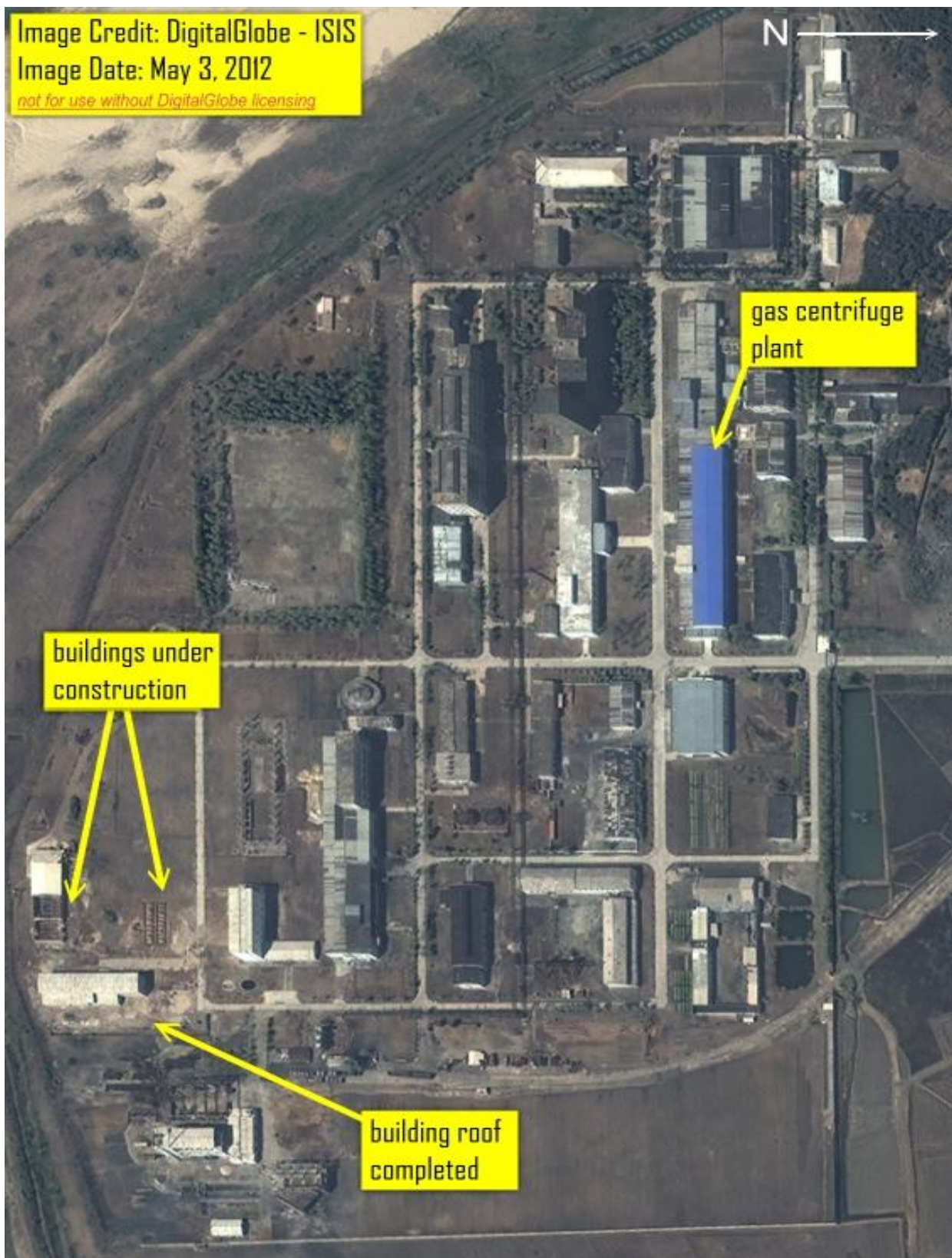
Figure 3. Digital Globe imagery from May 3, 2012 showing building construction in what is the south eastern corner of the fuel fabrication facility. Note the empty space between the centrifuge plant building that in the recent imagery has been covered by an extension to the plant building.
