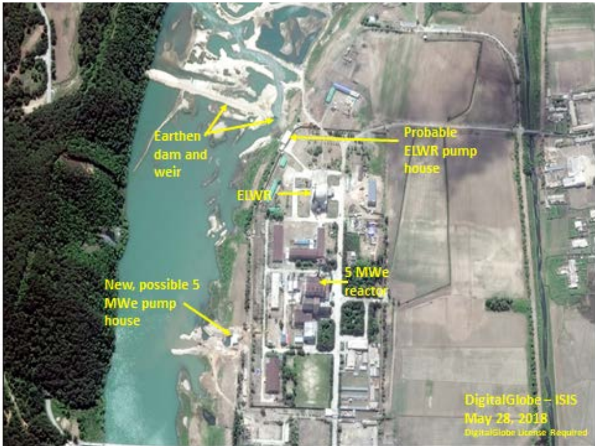
Figure 3. A recent satellite image indicates that the changes made at the Kuryong river bed likely serve the purpose of improving the two reactors' cooling systems.
