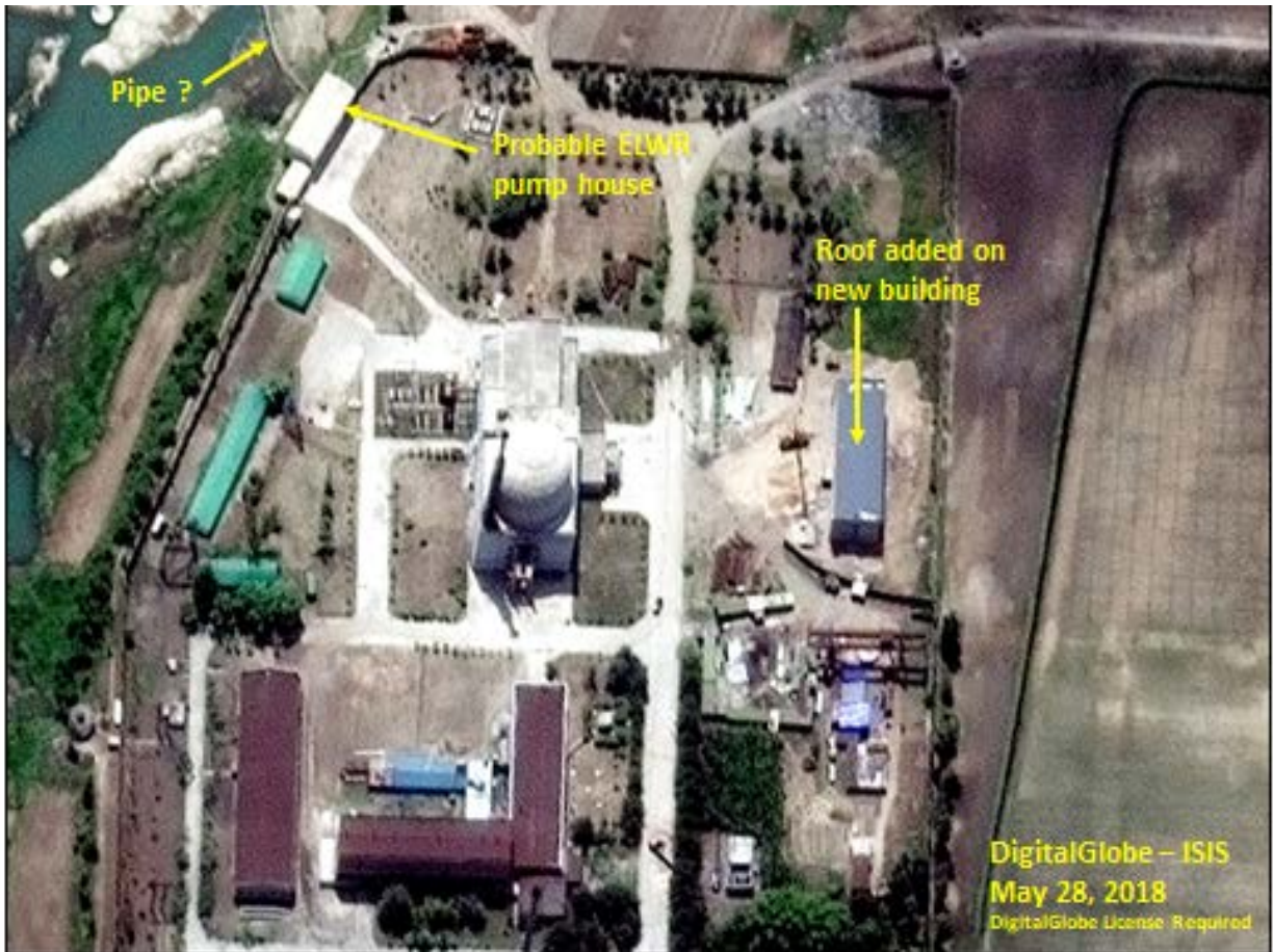
Figure 5. A new building added outside the ELWR’s main entrance seems to be near external completion.
