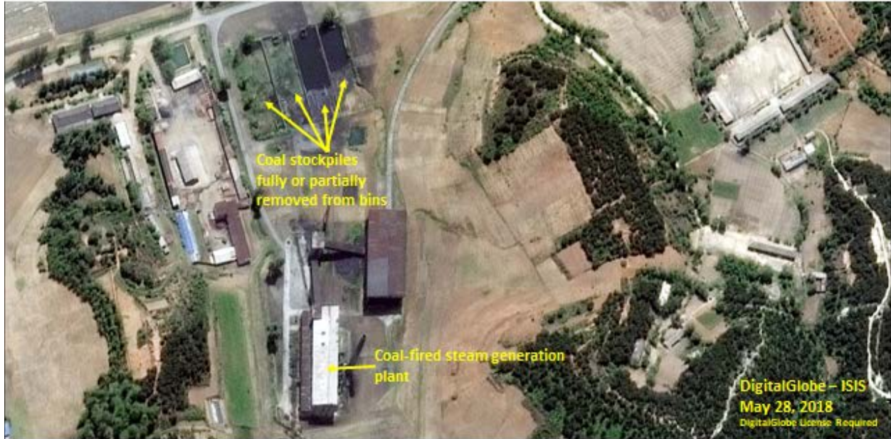
Figure 1. Compared to a May 6, 2018 DigitalGlobe image published and annotated by 38North , it appears that coal at the coal-fired thermal plant has been fully or partially removed from the individual stockpiles. No smoke is coming from the stack, indicating that the reprocessing campaign may have ended or been completed. The coal-fired plant supplies steam for operations at the Radiochemical Laboratory where reprocessing occurs.
