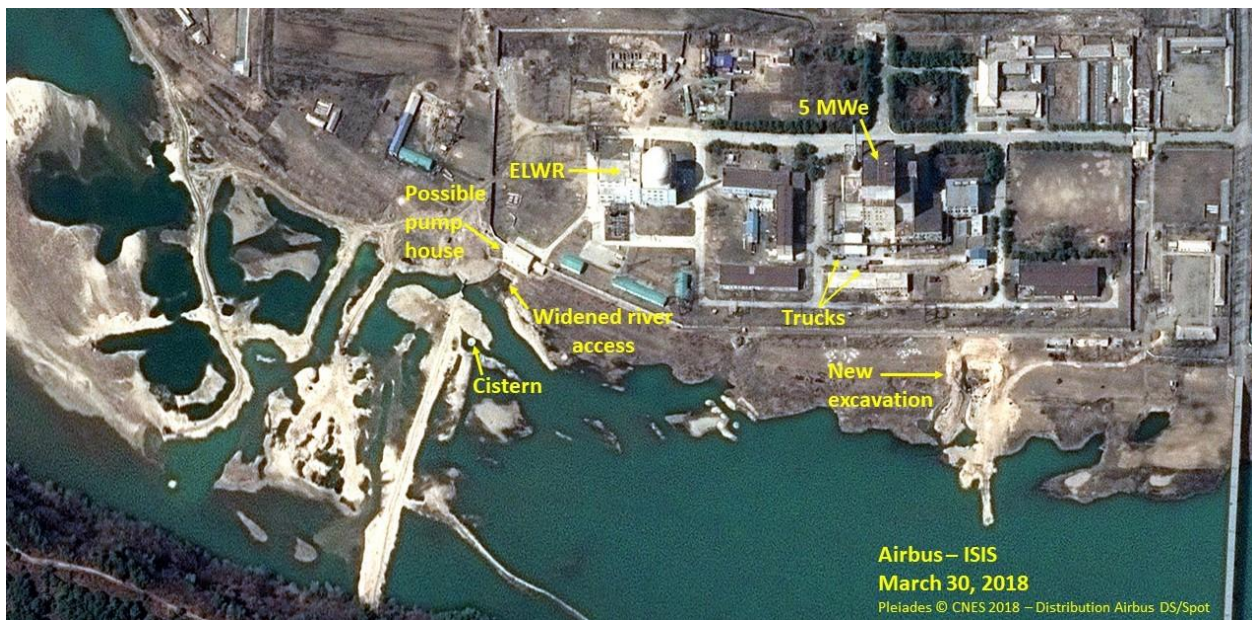
Figure 5. Widened water access below the probable pump house may serve to facilitate water intake or outflow for the reactor. The water in the immediate area is noticeably discolored, possibly indicating water movement or flow, the direction of which cannot be determined.
