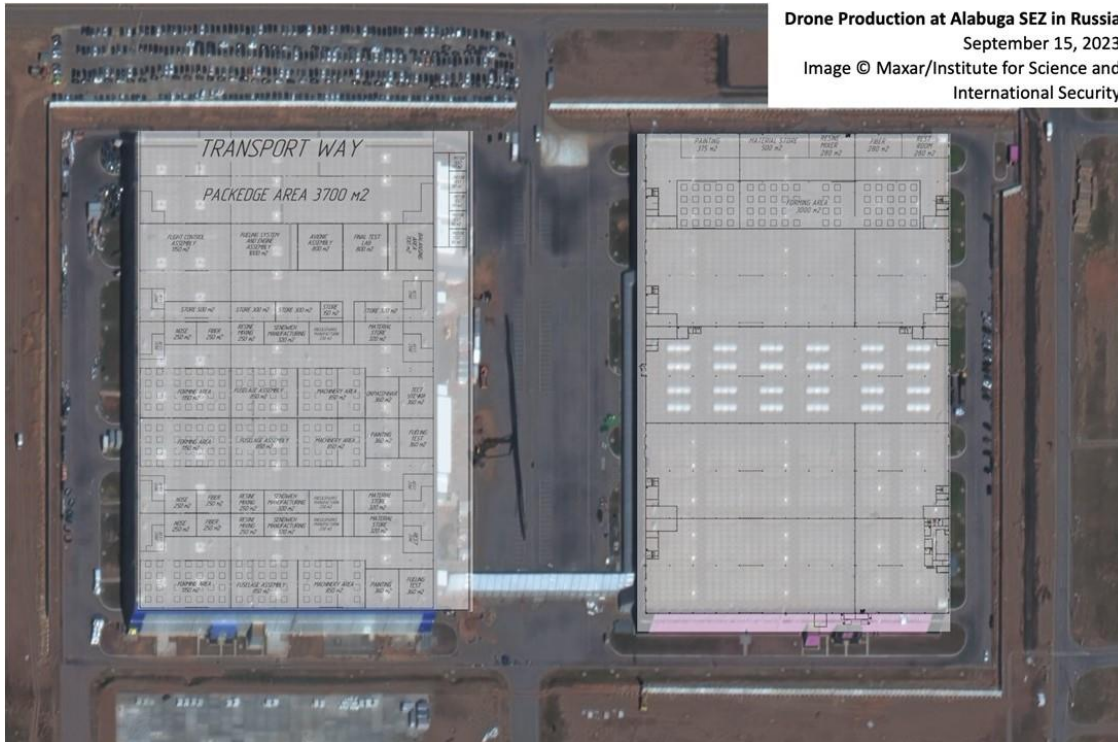
Figure 2. Overlay of floor plans for building 8.2 (left) and 8.1 (right) from internal Alabuga documents on recent satellite imagery shows that the buildings' dimensions and features match the layouts precisely.
