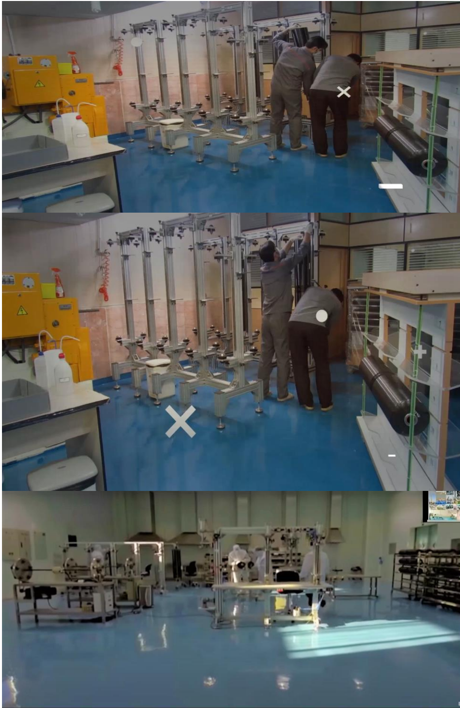
Figure 12. The top two photos show two workers loading an IR-6 assembled rotor vertically into a rotor straightening and balancing rig. Three or four rotor assemblies are visible in the photo. There are 20 rigs in total, some with different heights. The two personnel may be working with more than one rig at the same time. The workers must ensure that the rotor assembly is straight, which can be done by slowly rotating the assembly, while using probes and simple adjustments. For comparison, the bottom photo is of a similar, albeit far larger, room in the destroyed Iran Centrifuge Assembly Center, showing straightening and balancing equipment and rigs, racks of rotor tubes, and workers in protective, sanitary clothing. Such clothing is absent from personnel in the video, perhaps consistent with staged activities conducted for the video.
