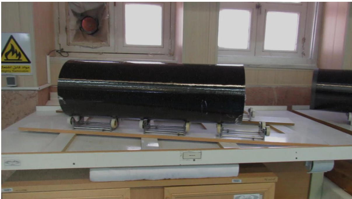
Figure 8. IR-6 rotor tubes on two adjacent work surfaces shown in consecutive freeze frames, panning from right to left. The top photo shows that the end of one rotor tube has been partly machined, likely for fitting purposes, and the other end holds a domed end cap (the machined end can also be seen in the partial rotor tube on the right side of the bottom image.) Accepting that the cylinder diameter is 200 millimeters then one can roughly measure the length from the photo as about 600 millimeters, as expected). Note that in the top image there are two domed top caps on the table awaiting to be fitted onto the cylinders. The caps appear to be made from carbon fiber and have a metal insert. The windows are consistent with being in a half-basement, such as found in the Natanz administration building (see text).
