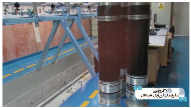
**Figure 16.** Three IR-6 test stands, with "case and base," are awaiting to be lowered into a test pit.
