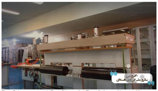
**Figure 3**. In same room as in Figure 2, two carbon fiber cylinders awaiting assembly. Between them is possibly a metal bellows, most logically made of maraging steel because of the relatively high speeds achieved by the advanced centrifuges.
