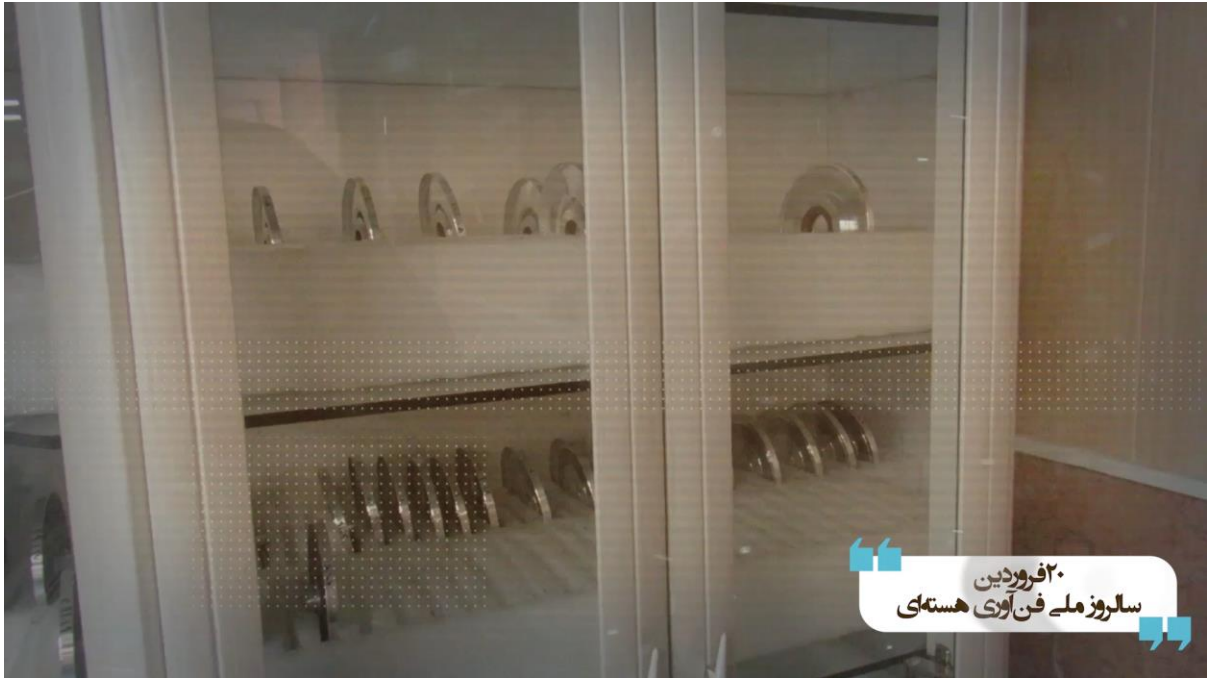
Figure 5. This cabinet contains a stock of centrifuge subcomponents. At first glance, they look like baffles made from metal rather than carbon fiber. Baffles are inserted in the rotor to create the counter-current gas flow and to isolate the top scoop extraction chamber. Note that the subcomponent is made of metal and not a carbon composite, and is likely made of maraging steel or high strength aluminum. They could also be end caps made out of high strength aluminum, where they are inserted inside the carbon fiber rotor tube, providing strengthening.
