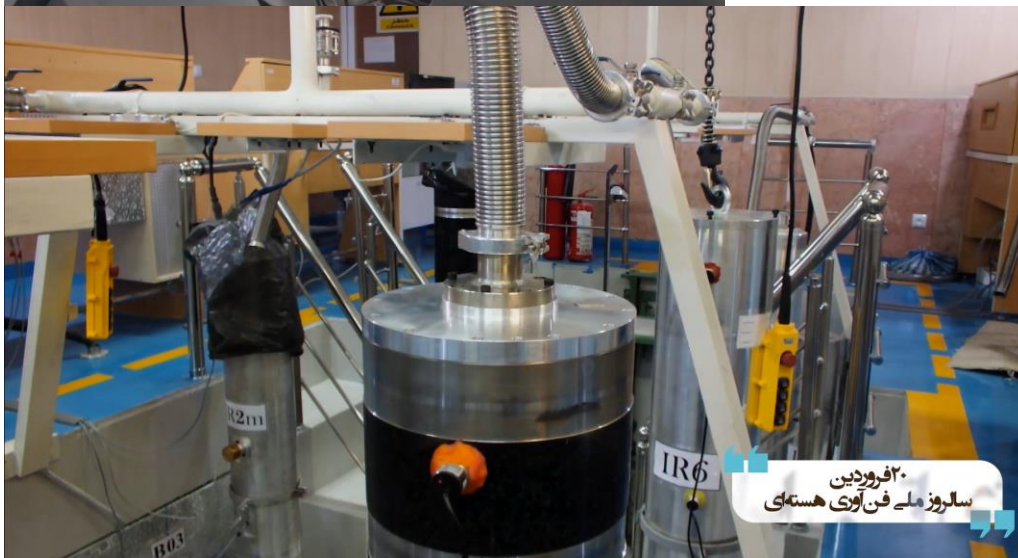
Figure 19. Top two images show close-ups of centrifuge test stands in a pit, labeled as the IR-6 centrifuge. Note that to the left of the IR-6 is an IR-2m machine test stand and to the right and slightly behind may be a version of an IR-6 machine with an aluminum outer casing rather than carbon steel. In the bottom photo, the IR-6 centrifuge is connected to vacuum piping and may be undergoing spin testing. The pit is marked B03, possibly related to location, and is not the same pit as in earlier images. In addition, the water coils appear to be missing. The labelling may reflect their use in other public videos released by the AEOL.
