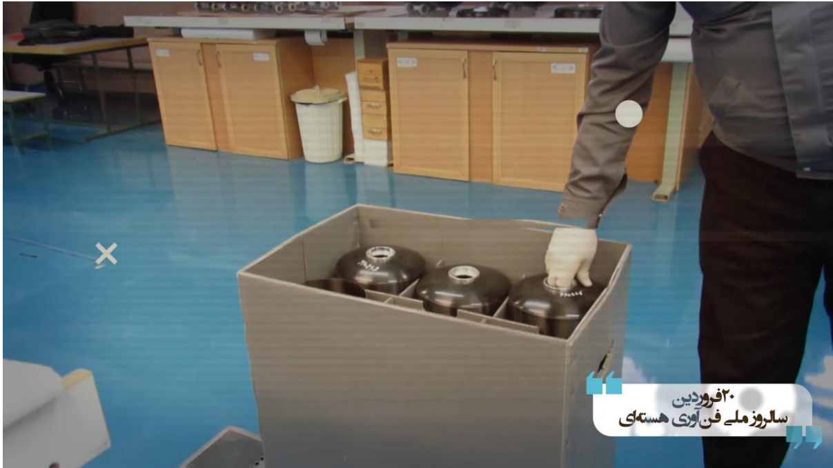
Figure 10. Visible is a carton box large enough for containing IR-6 rotor tubes and top caps. The top caps are domed with a flat section in the middle. Using the man's leg as a guide, the box appears to be about 800 millimeters in depth. Note that the end caps do not have rotating magnets installed at this point, although they look like they have a metal insert to hold the magnet. (The magnet holder, absent the magnet, may be used to hold the rotor vertically while checking its balance and straightness (see below.))
