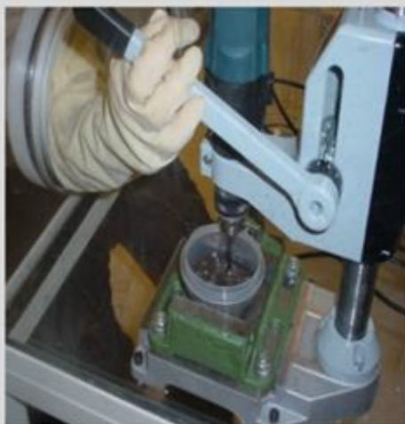
A drilling machine in a glove box
