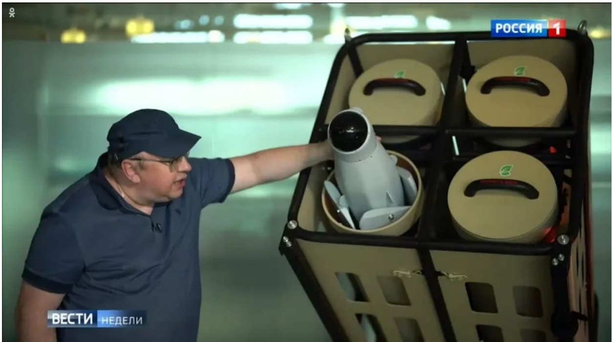
Figure 4. The four-tube launcher used to deploy the next generation Lancet drone, the Izdeliye-53.
