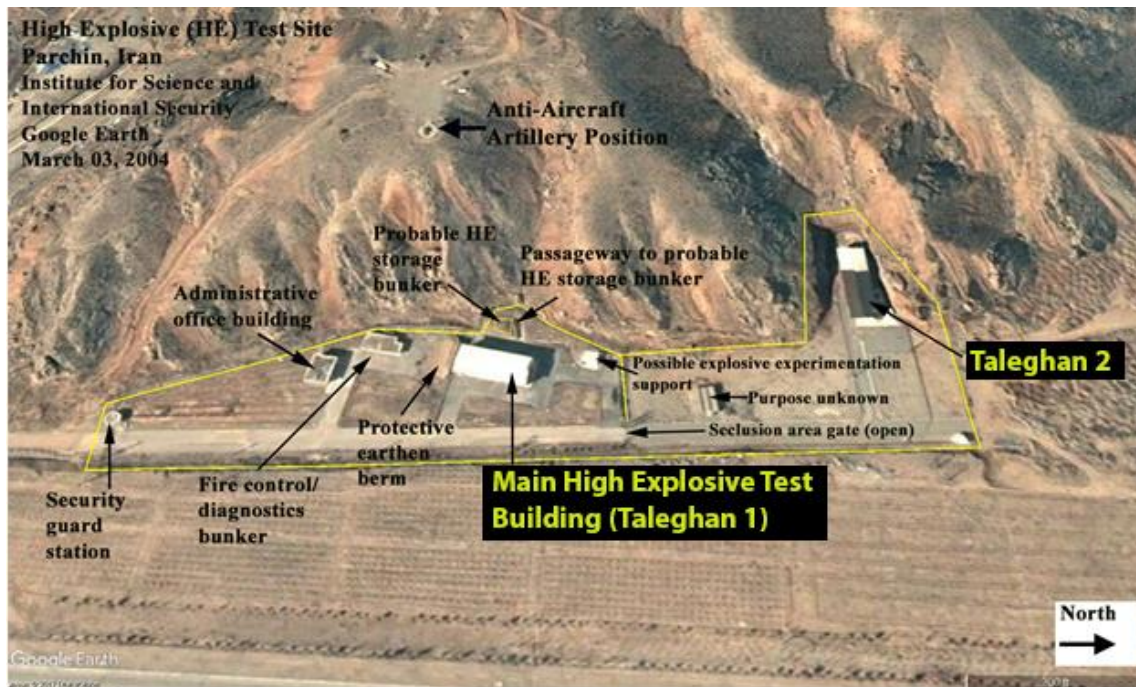
Figure 3. A 2004 Google Earth satellite image shows the Parchin complex that was involved in nuclear weapons high explosive testing under the “Amad Plan.” This site has been extensively sanitized by Iran. The Nuclear Archive contains extensive information on this site, in particular the two main facilities, which Iran calls in the documents Taleghan 1 and 2. Taleghan 1 contained the high explosive test chamber that is often discussed publicly, and Taleghan 2 contained a smaller high explosive test chamber and a flash x-ray system that was not visited by the International Atomic Energy Agency (IAEA).
