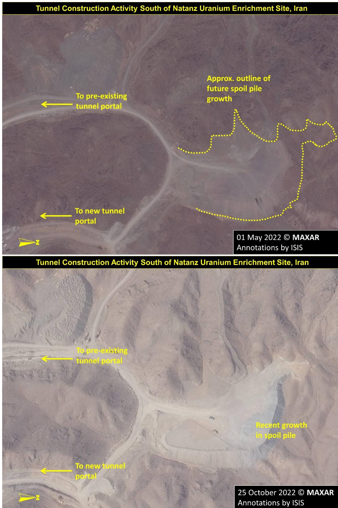
Figure 8. A comparison of the spoil pile near the western tunnel entrances from May 2022 (top) to October 2022 (bottom).
