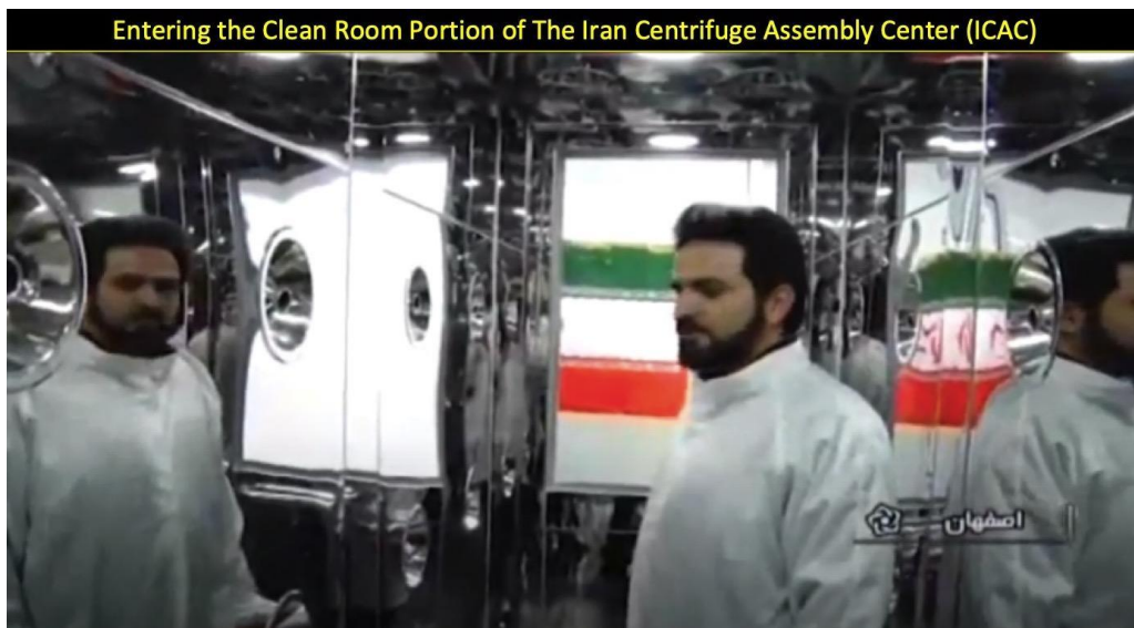
Figure 7. During a 2018 promotional video tour, a reporter is shown entering the portal to the clean room section of the ICAC. The lack of bonnets and facial hair coverings indicates that the clean room was not yet fully operational at that time.
