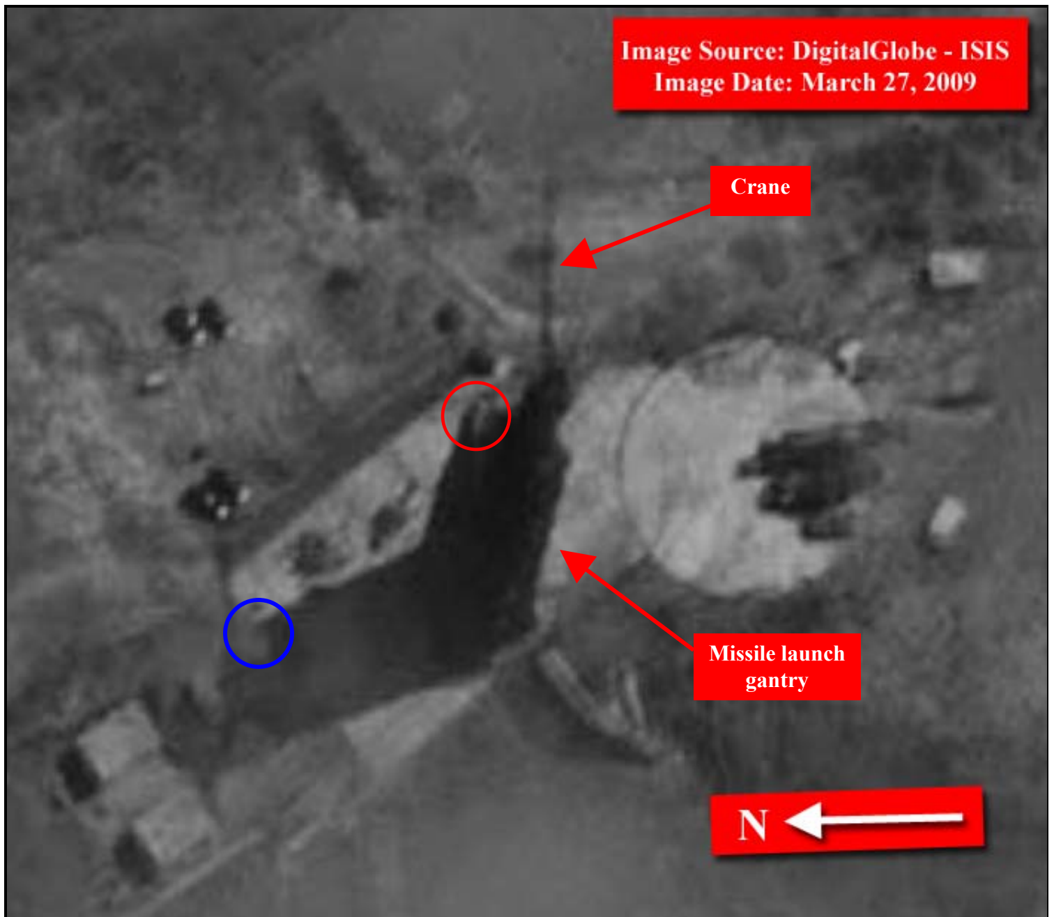
Figure 1. A close-up DigitalGlobe image of the launch pad at the Musudan-ri missile site on March 27, 2009. The red circle should be where the top of the missile would be located. The blue circle contains the shadow cast by the part of the gantry in the red circle. We could not determine if the light-colored area inside the red circle is the top of the missile.
