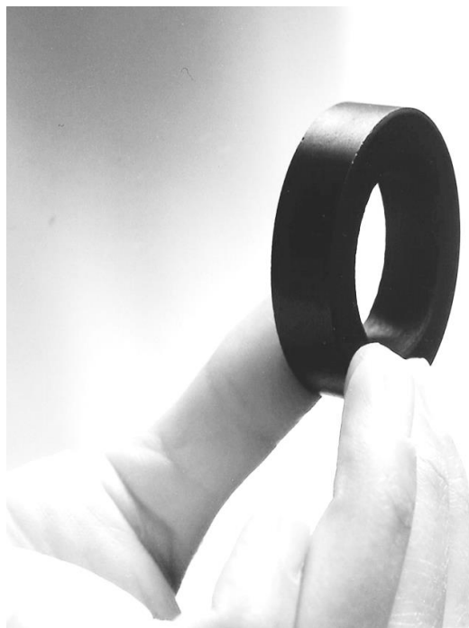
Figure 7 A ring magnet used in the top bearing of a centrifuge. Each top bearing uses two ring magnets. Iran obtained tens of thousands of ring magnets for its centrifuges abroad, particularly in Europe and China. It is unknown if Iran makes ring magnets for its centrifuges today or buys them abroad. The P5+1 and the IAEA should learn where Iran obtains ring magnets today and how many it has stockpiled for advanced centrifuges.
