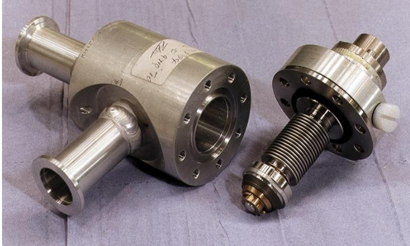
Figure 8 A vacuum bellows sealed valve showing subcomponents. On right is a convoluted tube, also called a bellows (which should not be confused with the bellows that is part of a rotor assembly). Iran's centrifuge program had thousands of these bellows made in China, in addition to vacuum valve housings, for its centrifuge program. After receiving the subcomponents, Iran assembled them into vacuum valves, including welding the bellows to the valve top. It is unknown if Iran continues to buy valve subcomponents abroad. The P5+1 and the IAEA should learn how and where Iran makes vacuum valves today and how much it depends on buying subcomponents from abroad.
