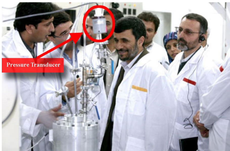
Figure 6 Then-President Mahmoud Ahmadinejad standing by an Iranian advanced centrifuge with a U.S.-manufactured pressure transducer, acquired by Iran illegally several years earlier. Iran cannot make reliable pressure transducers and acquired thousands of them abroad illegally. A critical question is determining how many of these and similar pressure transducers Iran acquired abroad and stockpiled. Credit: Iran's Presidential web site.
