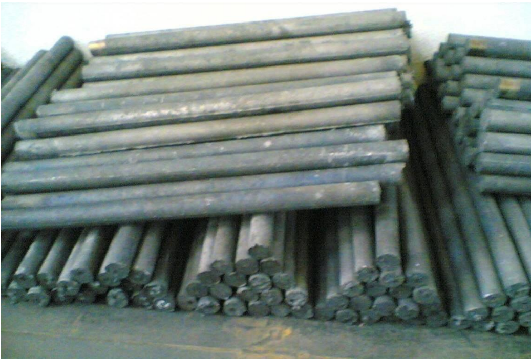
Figure 9: Image made available to ISIS of alleged natural uranium rods related to fuel in the Al Kibār reactor. The rough surface indicates the lack of cladding. The golden tips could suggest recent sampling that would have exposed the unoxidized metal.
