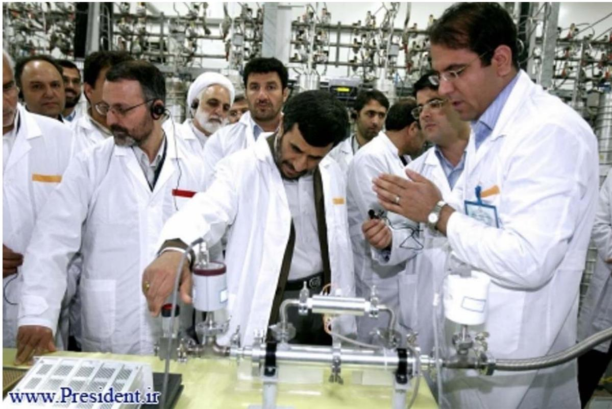
**Figure 3:** Former President Ahmadinejad examines gas centrifuge equipment, which includes an older MKS pressure transducer (next to his right hand) during a visit to the Natanz pilot fuel enrichment plant in 2008. In the background is an IR-1 gas centrifuge cascade which contains many more recent (mid-2000s) models of MKS pressure transducers. Source: Website archive of the president of Iran, [www.President.ir](http://www.President.ir)
