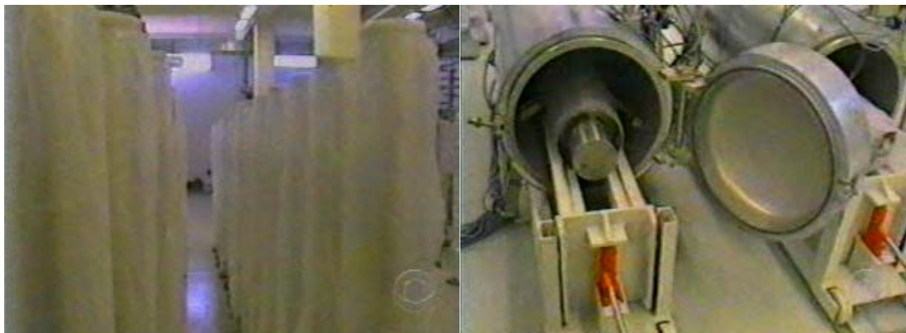
Figure 3: Inside the Al Hashan site that held P1 centrifuges, although Libya did not enrich any uranium before the program ended in 2003. On left, feed and withdrawal equipment, and on right, rows of unassembled P1 centrifuges. Photo credit: CBS 60 Minutes.
