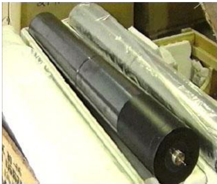
Figure 4: Two P2 centrifuge rotor assemblies. The one on the left shows a bellows in the middle of the tube and the pin of the bottom bearing, provided to Libya by the Khan network and subsequently sent to the United States. Photo Credit: NHK
