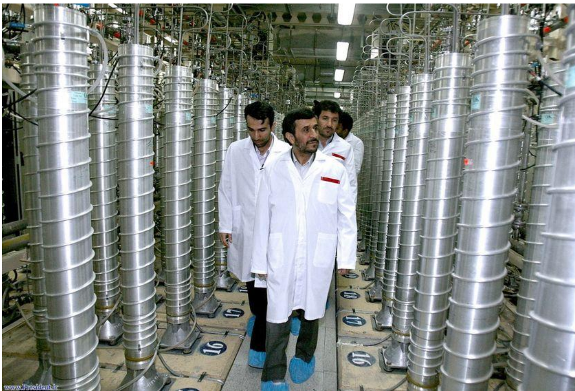
Figure 1: P1 centrifuges in the Iranian pilot enrichment plant at Natanz. They are organized into cascades, each containing 164 P1 centrifuges connected by pipes. Photo credit: photo archive of the web site of the President of Iran, www.president.ir .
