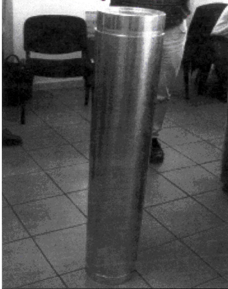
Figure 5: Outer casing of P2 centrifuge made at SCOPE in Malaysia.
