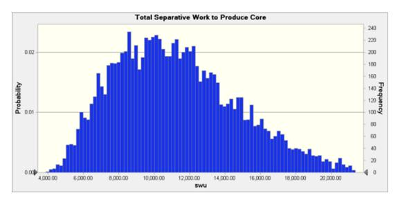
Figure 10. The separative work necessary to produce enough HEU for a submarine core.
