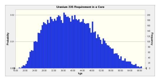
**Figure 9.** Amount of Uranium 235 initially in a naval core.
