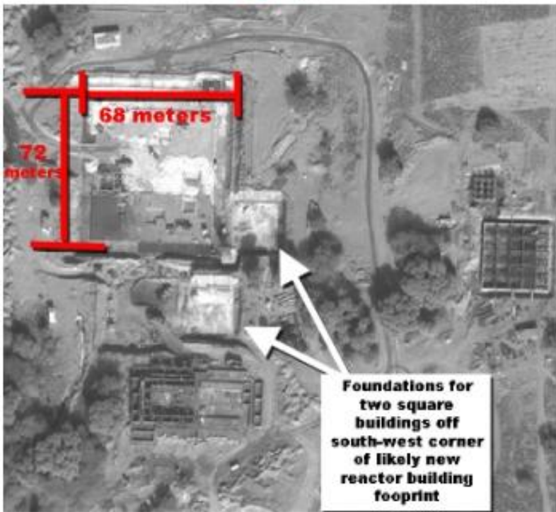
Figure 2. A comparison of the construction footprint of what is likely a new reactor seen in a January 15, 2011 image and the third Khushab reactor while it was under construction in a June of 2007 image. The dimensions of the third reactor building seen in 2007 and the footprint seen in January 2011 are nearly the same. The placement of two square buildings off the south-west corner of each building construction is also very similar.
