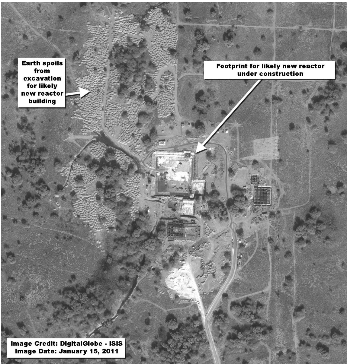
Figure 1. January 15, 2011 commercial satellite image showing the footprint for the likely new reactor under construction at the Khushab site.
