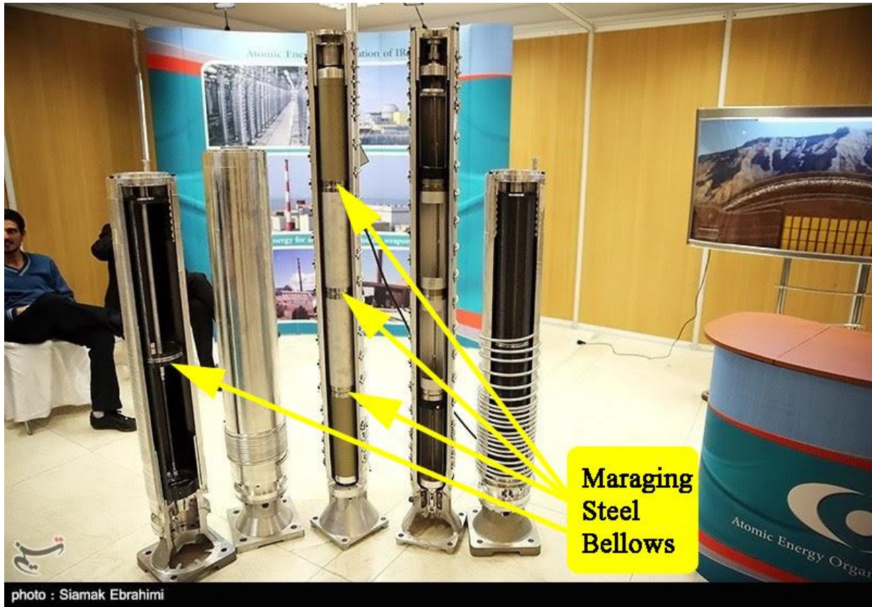
Figure 1. This image shows at least three Iranian centrifuges and bellows at a recent Atomic Energy Organization of Iran exhibition in Tehran. The centrifuges on the far left and far right appear to be IR-2m centrifuges, each of which has a rotor assembly with two carbon fiber rotors (black) connected by a thin maraging steel bellow. The IR-2m bellows are believed to be made from 350 maraging steel. The tall centrifuges in the middle are IR-1 centrifuges, each of which has a rotor assembly made from four high-strength aluminum rotor tubes and three maraging steel bellows. The IR-1 bellows may be made from 300 or 350 maraging steel. The second centrifuge from the left is of an unknown type; some have speculated it is an IR-4 centrifuge.
