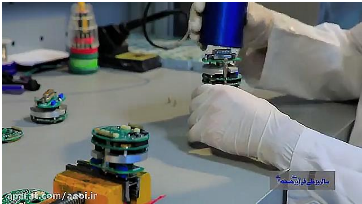
Figure 10. A worker enclosing a completed pressure transducer.
