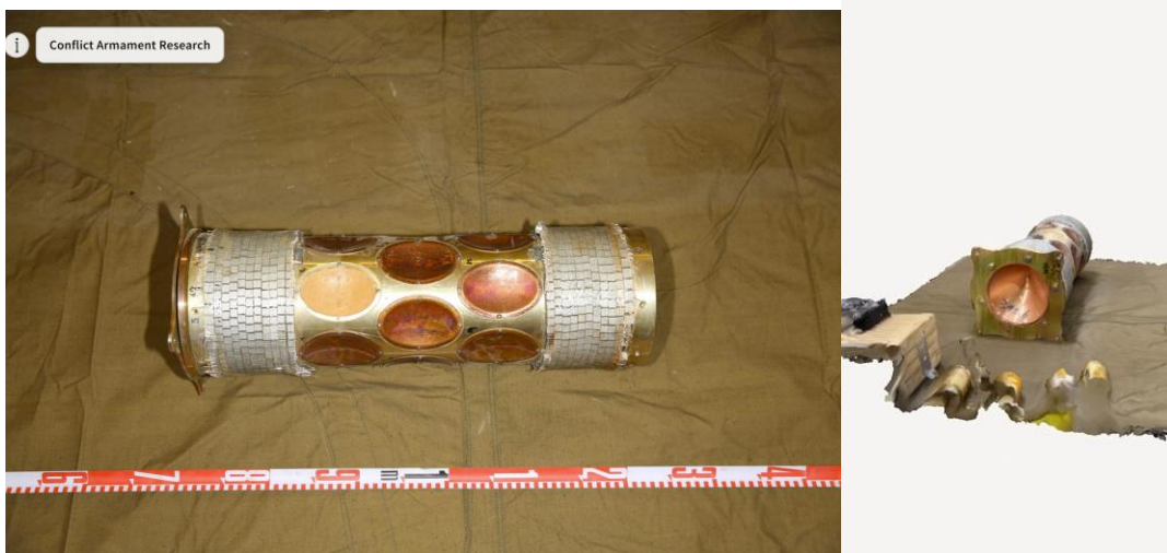
Figure 2. A multipurpose warhead from a Shahed 131 drone. The copper discs visible in the left image are used to create radial anti-armor effects. Two fragmentation belts composed of eleven layers of metal cubes (type not provided) are also visible in the left image. There is a primary cone-shaped liner in the forward section of the warhead (see right image), which corresponds to the copper funnel in the bumper's parts list. Source: Conflict Armament Research (see footnote 4).
