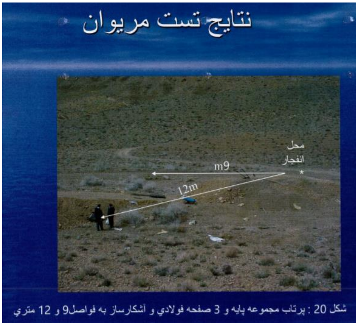
Figure 7. Slide 20 of the Nuclear Archive slide set titled “Marivan Test Results.” The caption reads, “The throwing of the set of the base and three steel plates and detector to the distances of 9 and 12 meters.”
