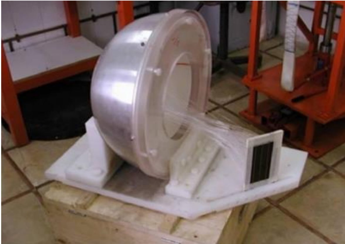
Figure 3. Model of an experimental system in the Nuclear Archive representing what appears to be a shock wave generator and high explosives, with a diagnostic system using fiber optic cables, to measure time of arrival of a detonation front in the main charge.
