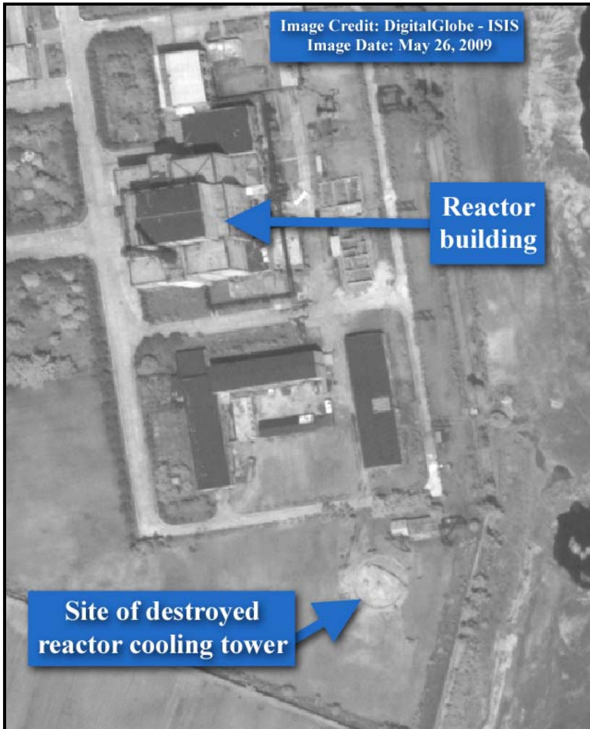
Figure 4. May 26, 2009 DigitalGlobe image showing the site of the destroyed cooling tower. There does not appear to be any construction activity near where the cooling tower had previously stood. North Korea imploded the cooling tower in June 2008 as a disablement measure.
